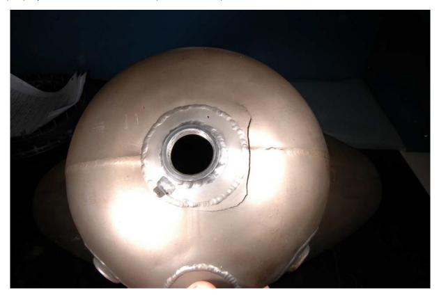
Allison: 250C47B, Cracked Combustion Case, ATA 7240
